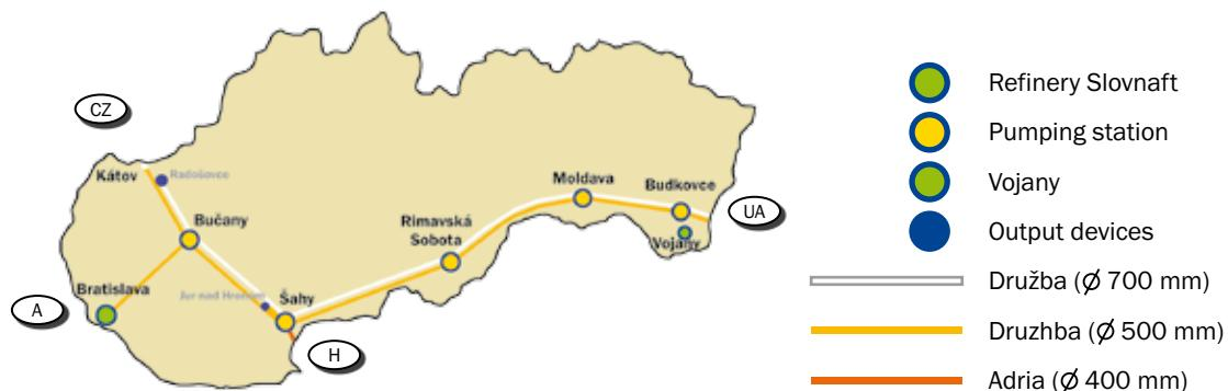
Fig. 2 The crude oil pipeline Družba in the SR.
